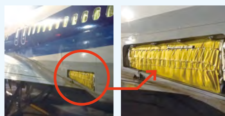
Boeing 767 With Missing Panel
